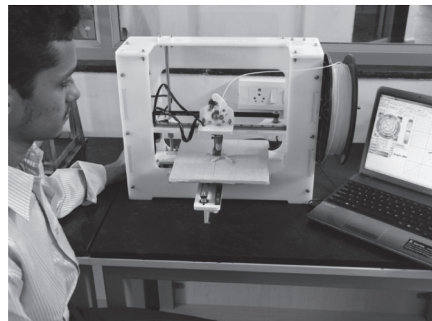
Fig. 1: Low-cost 3D Printer for automatic fabrication of plastic patterns.
